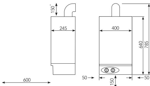
\*From casing or 25mm above flue elbow (whichever is applicable)
