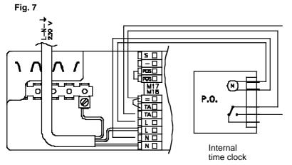
Fig. 7 Showing 230v input electrical connection and internal timer without room thermostat.
