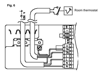
Fig. 6 Showing 230v input electrical connection and room thermostat connection (connected between TA & TA) without internal time clock. (Remove link between = & TA). Note: room thermostat contact rated at 230v. Should the room thermostat require a neutral or earth, connect neutral to one of the terminals marked N, and the earth to the earthing strip.
