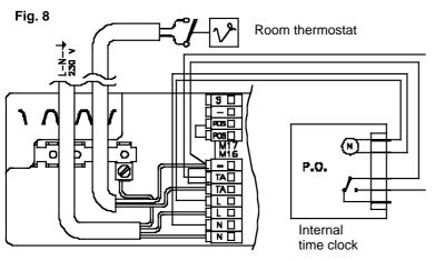
Fig. 8 showing 230v input electrical connection internal timer and room thermostat. Note:
