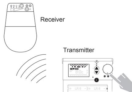
Ensure the transmitter has been set/left in the coding mode (menu > service > coding > OK) and press button B on the receiver for approximately 5-seconds, LED A will light up briefly. Press ESC to escape from the coding mode.
