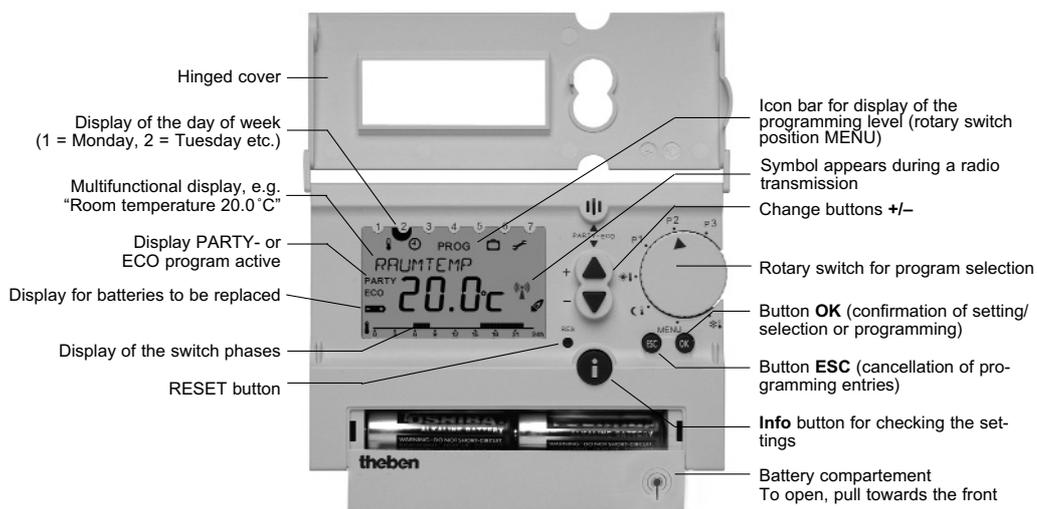
Once the batteries have been inserted into the battery compartment and the OTR has been connected to the boiler, the transmitter can be mounted/located and programmed for use.
