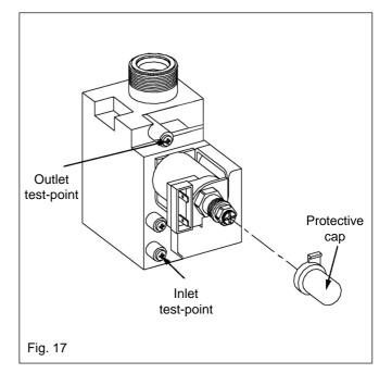
Once the burner pressure has been checked, isolate the appliance from the electrical supply, remove the manometer and tighten the gas valve outlet test nipple.
