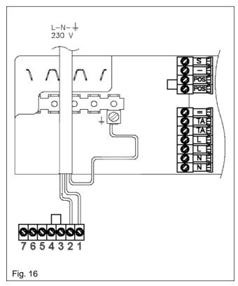
Connect the supply cable wires (LIVE and NEUTRAL) to their corresponding terminals on the appliance terminal block. Connect the EARTH wire to the EARTH block (see fig. 16) ensuring that it's left slightly longer that the others, this will prevent strain on the EARTH wire should the cable become taut.
