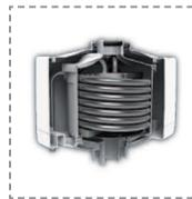
The post heat exchanger device is located between the boiler and flue terminal. The device offers the potential to increase efficiency by capturing some of the heat in boiler flue gases that would normally be wasted. It uses this extracted heat to reduce the amount of fuel that has to be burned when providing hot water.
