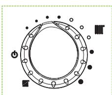
The central heating temperature can easily be adjusted using the heating temperature selector.
