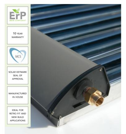
**TECHNICAL SPECIFICATIONS** Total area  $2.77 \text{ m}^2$ 2.40 m<sup>2</sup> Exposed area Effective absorption area 2.69 m<sup>2</sup> Dimensions (mm) (HxWxD) 1730 x 1600 x 145 Empty weight 52 kg Liquid content 2.05 litres Recommended flow rate of panel (per m<sup>2</sup>/h) 30 litres > 94% Absorption (a) Emissions (B) < 7% Maximum permitted pressure 10 bar Maximum temperature 236°C
