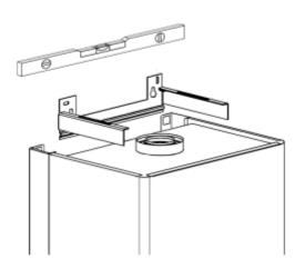
3. Mount the Fuelsaver on the support bracket and insert into the boiler flue spigot. Using the clamp, gasket, and screws supplied, secure the Fuelsaver to the boiler.
