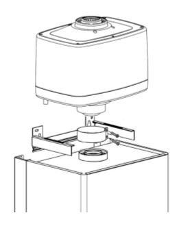
Always take into account the installation of the flue system. We recommend making the hole in the wall first but if the boiler is already installed, efforts must be made to cover the boiler during drilling to prevent debris falling into the appliance.
